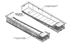
For sectionalized construction pools are pre-assembled in large sections for minimal assembly on-site. A section consists of floor, walls and structure welded together in house. Equipment is required for sections to get to the pool area as well to maneuver once in the pool. Oversized freight charges may apply depending upon sizes of sections. This further reduces on-site time over unitized/panelized construction.
